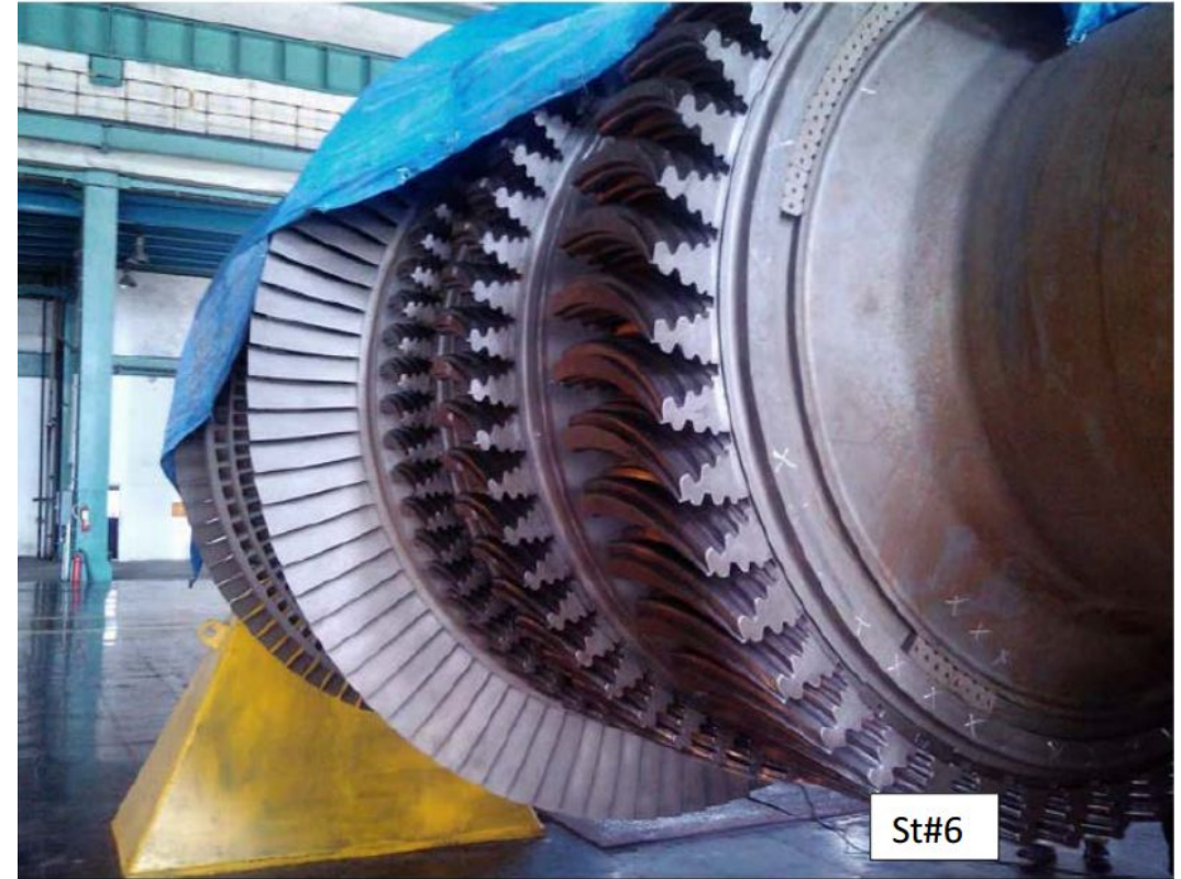
LP Rotor: Fir Tree Grooves (Axial entry)
